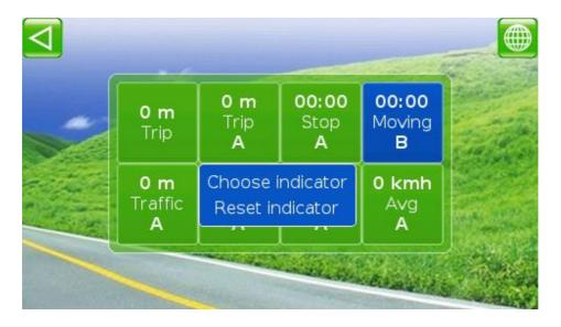
To customize the indicator, tap it. To set the readings to zero, select **ZERO THE INDICATOR**
