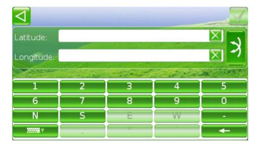
This function is designed for searching points by precise setting of their location within one of coordinate systems.
