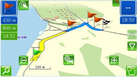
**Example:** When the route is selected and you need to continue movement after final point to the next one, select the point or place required and tap this button. The route will be prolonged to this point. The previous final point will be indicated as a passing one.
