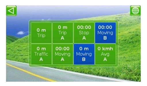
The Trip Computer provides information from indicators, and allows to customize the list of indicators. To open the trip computer, tap **TRIP COMPUTER** in the Main Menu.
