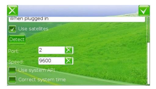
Sequentially fill in all symbols of the port number in the field **PORT** and its speed - in the field **SPEED**. Tap
